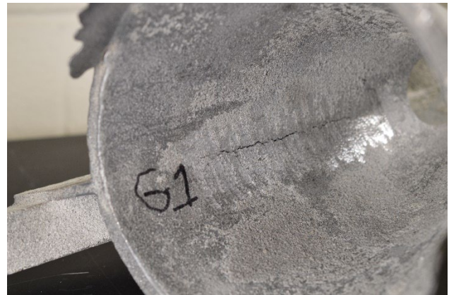
Figure 12. Typical hot tear in WCB casting.
