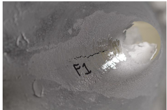
Figure 13. Typical hot tear in Med-Mn steel.
